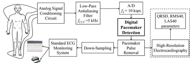
Figure 1. Overall block diagram of a possible ECG system
