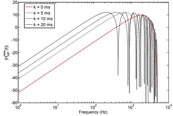
Figure 3. Magnitude of the linear filter frequency response.
