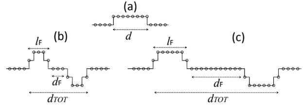
Figure 2. (a) ideal pacing pulse; (b) filtered signal  $s_{HP}^{new}[n]$  with  $k < d$ ; (c) filtered signal  $s_{HP}^{new}[n]$  with  $k > d$
