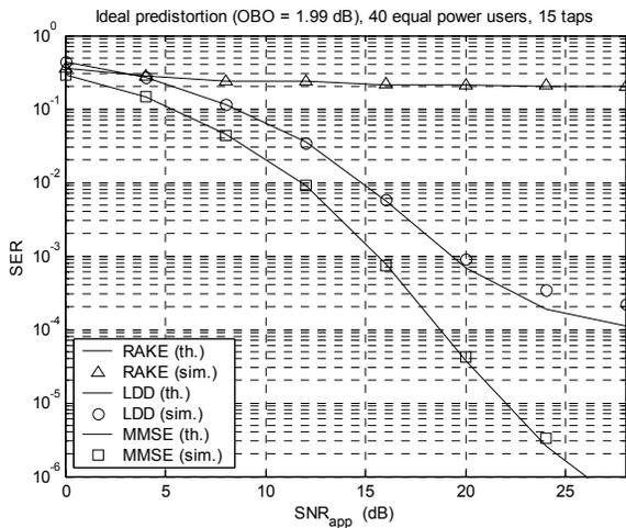
Fig. 2. SER comparison in frequency-selective channels.
