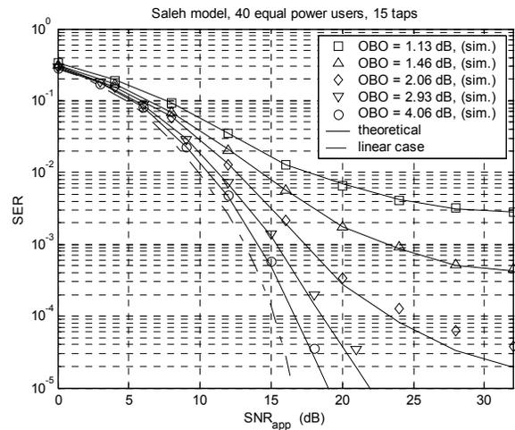
Fig. 4. SER of the MMSE in frequency-selective channels.
