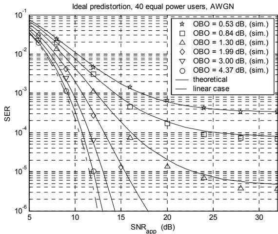
Fig. 1. SER of the MMSE detector in AWGN channels.
