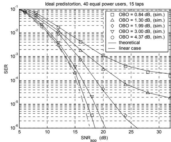
Fig. 3. SER of the MMSE in frequency-selective channels.
