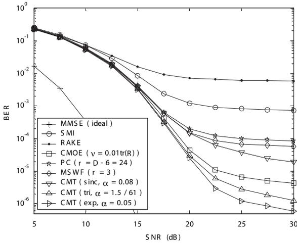
Fig. 1. BER comparison of various detectors as a function of the SNR.
