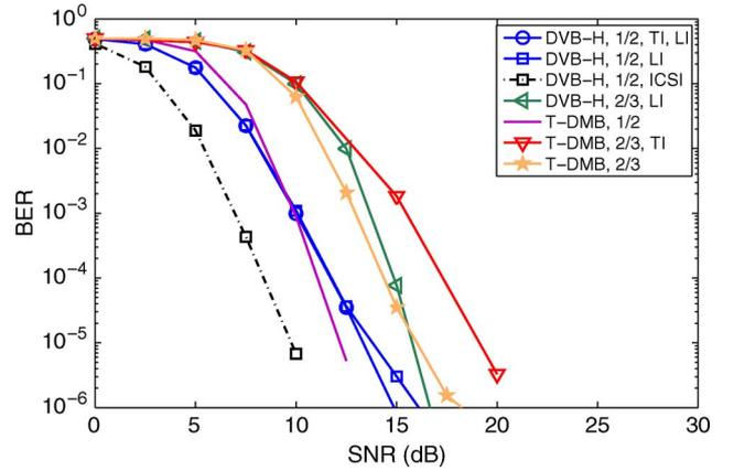
Fig. 1. BER performance of DVB-H at 8 MHz and T-DMB, at the output of the Viterbi decoder (inner BER, i.e., excluding outer RS coding). Rayleigh BU channel,  $f_C = 800$  MHz,  $v = 150$  km/h ( $\bar{f}_D = 0.019$  for T-DMB,  $\bar{f}_D = 0.025$  for DVB-H). For TI cases,  $v = 0$  km/h.
