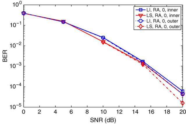
Fig. 5. BER performance of DVB-H at 8 MHz, at the output of the Viterbi decoder (inner) and of the outer RS decoder. Convolutional CR  $r = 1/2$ , Rice RA channel with  $K = 0$  dB,  $f_C = 800$  MHz,  $v = 150$  km/h ( $\bar{f}_D = 0.025$ ).
