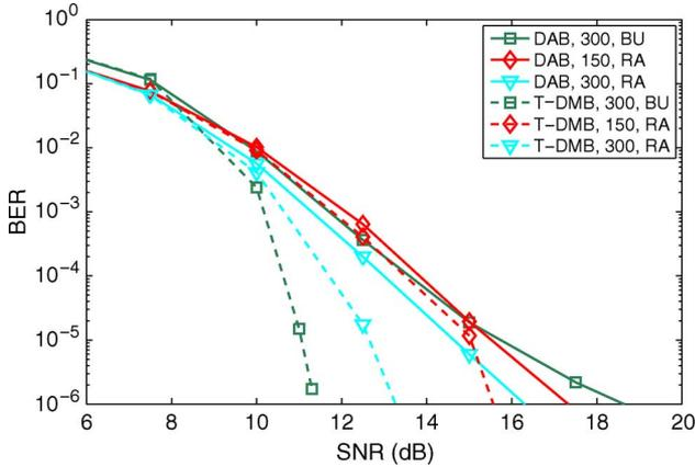
Fig. 9. BER performance of T-DMB at the output of the Viterbi decoder (DAB) and of the outer RS decoder. Rayleigh BU or Rice RA channel with  $K = 0$  dB,  $f_C = 1.4$  GHz,  $\mathbf{CR} r = 1/2$ ,  $v = 150$  km/h ( $\bar{f}_D = 0.034$ ) and  $v = 300$  km/h ( $\bar{f}_D = 0.067$ ).
