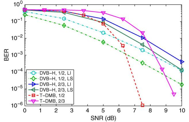
Fig. 7. BER performance of DVB-H at 5 MHz and T-DMB, at the output of the outer RS decoder. Rice RA channel with  $K = 10$  dB,  $f_C = 1.4$  GHz,  $v = 150$  km/h ( $\bar{f}_D = 0.034$  for T-DMB,  $\bar{f}_D = 0.070$  for DVB-H).
