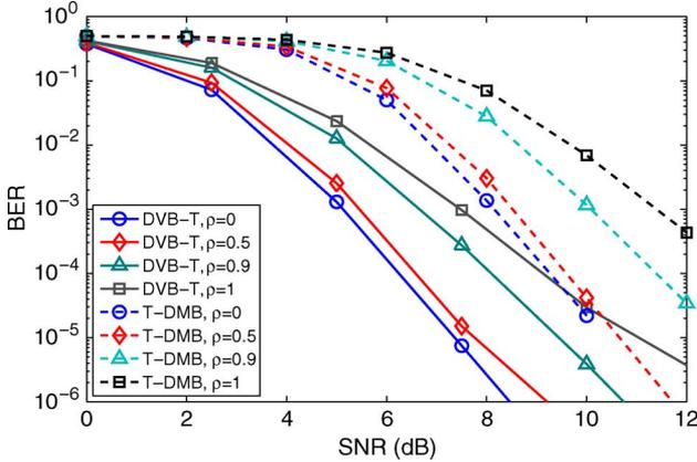
Fig. 12. BER performance of DVB-T at 8 MHz with  $r = 1/2$  and T-DMB (DAB) with  $r = 2/3$  at the output of the Viterbi decoder, for two receive antennas. **Rayleigh BU** channel,  $f_C = 800$  MHz,  $v = 300$  km/h ( $\bar{f}_D = 0.038$  for T-DMB,  $\bar{f}_D = 0.050$  for DVB-T).
