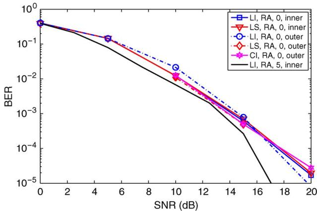
Fig. 6. BER performance of DVB-H at 8 MHz, at the output of the Viterbi decoder (inner) and of the outer RS decoder. Convolutional CR  $r = 1/2$ , Rice RA channel with  $K = 0$  dB or  $K = 5$  dB,  $f_C = 800$  MHz,  $v = 300$  km/h ( $\bar{f}_D = 0.050$ ).
