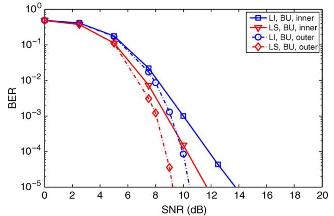
Fig. 3. BER performance of DVB-H at 8 MHz, at the output of the Viterbi decoder (inner) and of the outer RS decoder. Convolutional CR  $r = 1/2$ , Rayleigh BU channel,  $f_C = 800$  MHz,  $v = 150$  km/h ( $\bar{f}_D = 0.025$ ).
