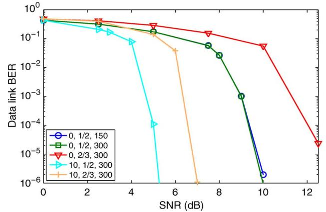
Fig. 11. DL layer BER performance of DVB-H at 8 MHz at the output of the MPE-FEC decoder. Rice RA channel with  $K = 0$  dB or  $K = 10$  dB,  $f_C = 1.4$  GHz, convolutional  $\mathbf{CR} r = 1/2$  or  $r = 2/3$ ,  $v = 150$  km/h ( $\bar{f}_D = 0.025$ ) or  $v = 300$  km/h ( $\bar{f}_D = 0.050$ ).
