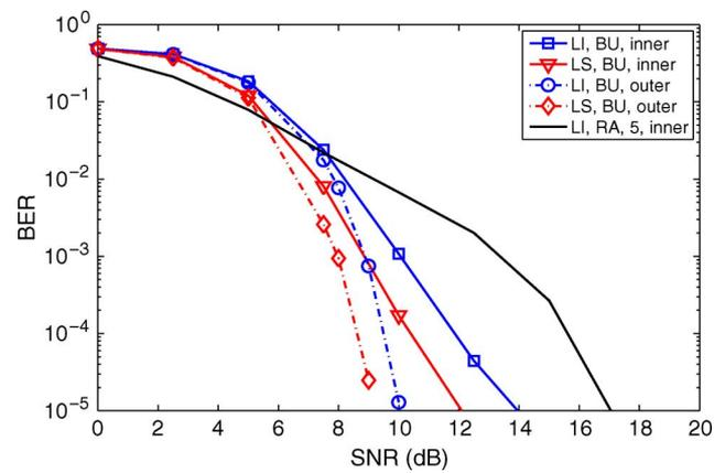
Fig. 4. BER performance of DVB-H at 8 MHz, at the output of the Viterbi decoder (inner) and of the outer RS decoder. Convolutional CR  $r = 1/2$ , Rayleigh BU or Rice RA channel with  $K = 5$  dB,  $f_C = 800$  MHz,  $v = 300$  km/h ( $\bar{f}_D = 0.050$ ).
