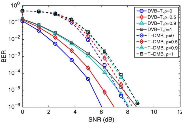
Fig. 13. BER performance of DVB-T at 8 MHz with  $r = 1/2$  and T-DMB (DAB) with  $r = 2/3$  at the output of the Viterbi decoder, for two receive antennas. **Rice RA** channel with  $K = 10$  dB,  $f_C = 800$  MHz,  $v = 300$  km/h ( $\bar{f}_D = 0.038$  for T-DMB,  $\bar{f}_D = 0.050$  for DVB-T).
