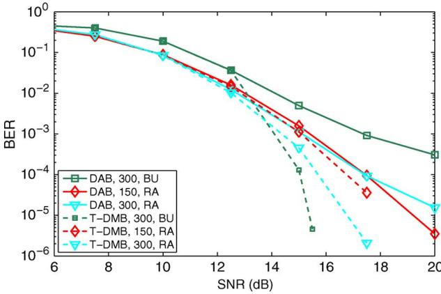
Fig. 10. BER performance of T-DMB at the output of the Viterbi decoder (DAB) and of the outer RS decoder. Rayleigh BU or Rice RA channel with  $K = 0$  dB,  $f_C = 1.4$  GHz,  $\mathbf{CR} r = 2/3$ ,  $v = 150$  km/h ( $\bar{f}_D = 0.034$ ) and  $v = 300$  km/h ( $\bar{f}_D = 0.067$ ).
