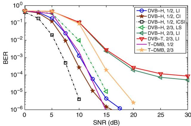
Fig. 2. BER performance of DVB-H at 8 MHz and T-DMB, at the output of the Viterbi decoder (inner BER, i.e., excluding outer RS coding). Rayleigh BU channel,  $f_C = 800$  MHz,  $v = 300$  km/h ( $\bar{f}_D = 0.038$  for T-DMB,  $\bar{f}_D = 0.050$  for DVB-H).
