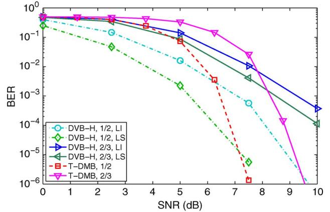
Fig. 8. BER performance of DVB-H at 5 MHz and T-DMB, at the output of the outer RS decoder. Rice RA channel with  $K = 10$  dB,  $f_C = 1.4$  GHz,  $v = 300$  km/h ( $\bar{f}_D = 0.067$  for T-DMB,  $\bar{f}_D = 0.139$  for DVB-H).
