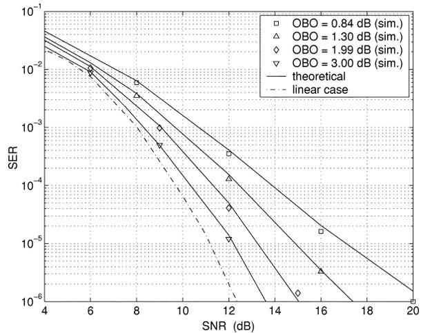
Fig. 7. SER of the mmse in frequency-selective channels (soft limiter,  $K = 20$ ).
