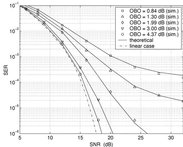
Fig. 5. SER of the mmse in frequency-selective channels (soft limiter,  $K = 40$ ).
