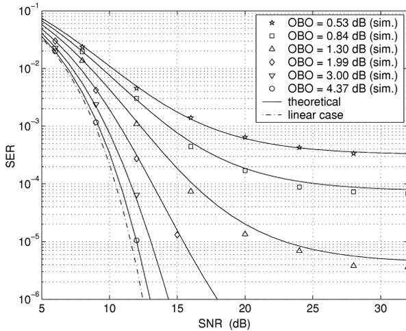
Fig. 1. SER of the mmse detector in AWGN channels (soft limiter  $K = 40$ ).
