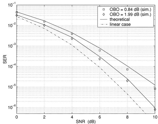
Fig. 8. SER of the mmse in frequency-selective channels (soft limiter  $K = 10$ ).
