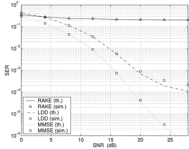
Fig. 3. SER comparison in frequency-selective channels (soft limiter, OBO = 1.99 dB,  $K = 40$ ).
