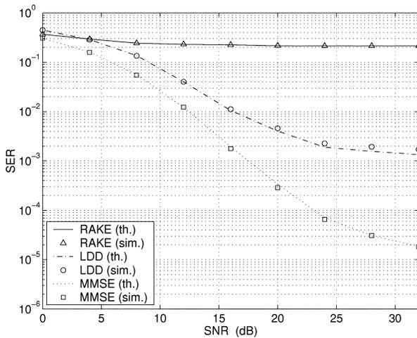
Fig. 2. SER comparison in frequency-selective channels (soft limiter, OBO = 1.30 dB,  $K = 40$ ).
