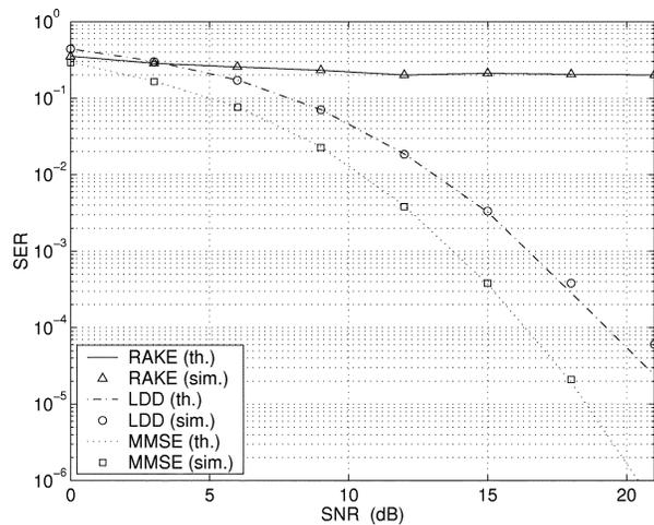
Fig. 4. SER comparison in frequency-selective channels (soft limiter, OBO = 3.00 dB,  $K = 40$ ).
