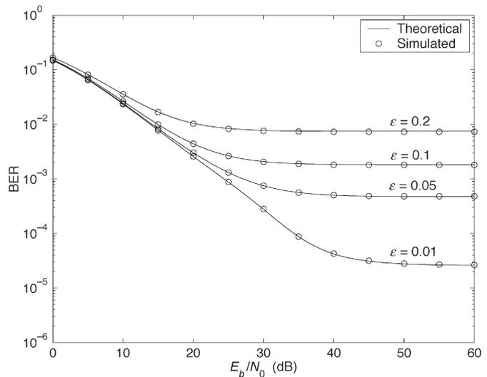
Fig. 4. BER of QPSK in the presence of guard bands.
