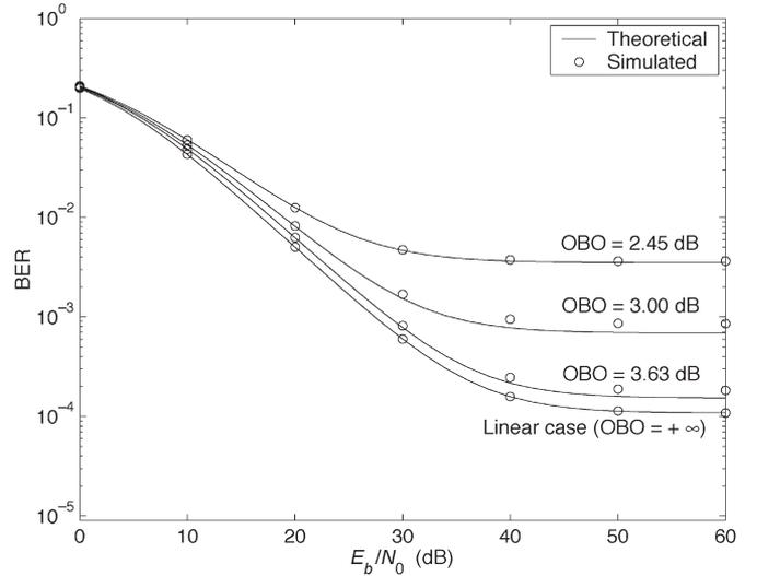
Fig. 7. BER of 16-QAM in the Rayleigh channel B when  $\varepsilon = 0.01$ .
