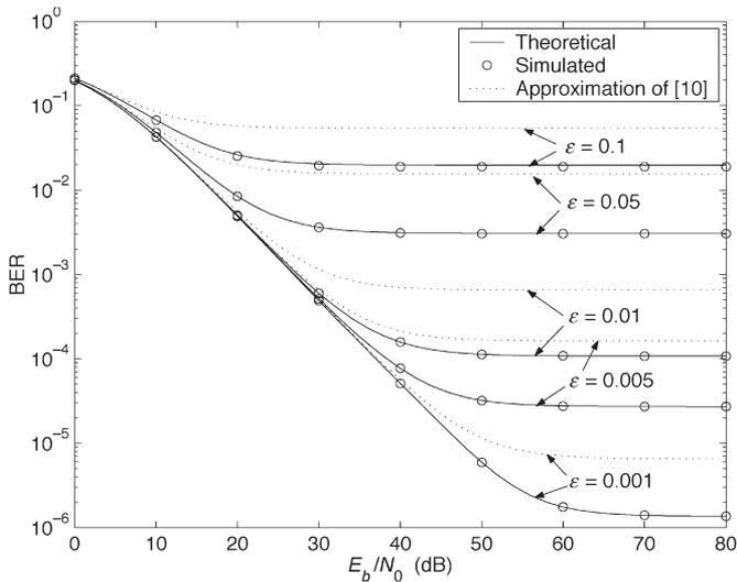
Fig. 2. BER of 16-QAM in the Rayleigh channel B.
