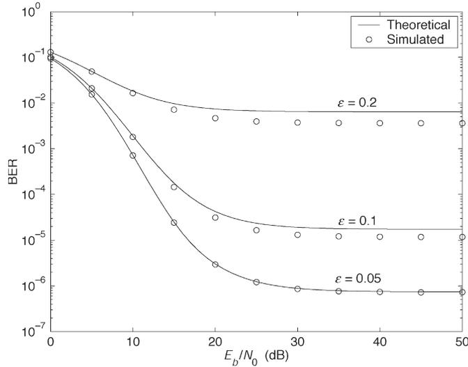
Fig. 5. BER of QPSK in the Rician channel D.
