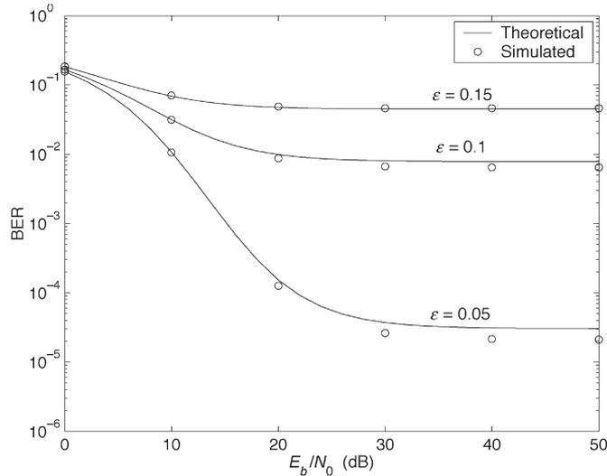
Fig. 6. BER of 16-QAM in the Rician channel D.
