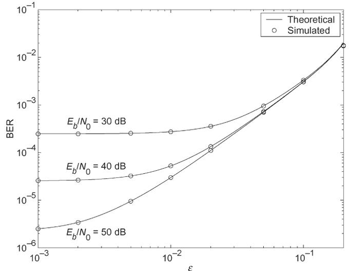
Fig. 3. BER of QPSK in the Rayleigh channel B.
