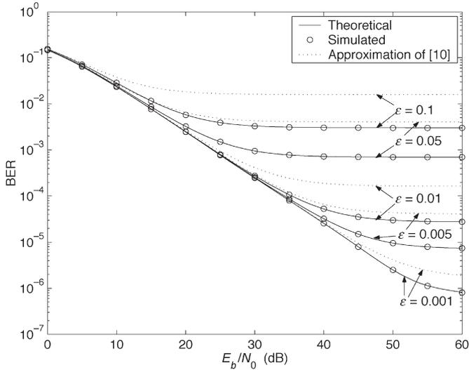
Fig. 1. BER of QPSK in the Rayleigh channel B.
